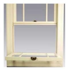
To tilt the top sash, lower the sash about half way. Pull the tilt latches (in the top edge of sash top rail) simultaneously until they clear unit frame when tilting. Ease top of sash toward you to a horizontal position.
