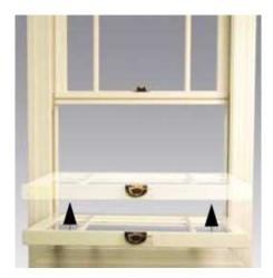
Now rotate the sash until pivot pins clear the jambs and remove the bottom sash from the frame.
